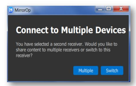
If you select "Multiple", MirrorOp Sender will connect to the second receiver and keeps the connection with the first one. You can see there are two check marks on the list now. Repeat the procedure if you want to connect to more receivers simultaneously.
