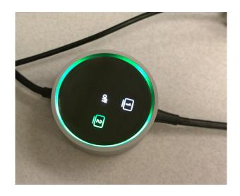
Use the puck connected to your computer to select which monitor you would like to display your screen to. You can display to 1 or 2 screens at a time.
